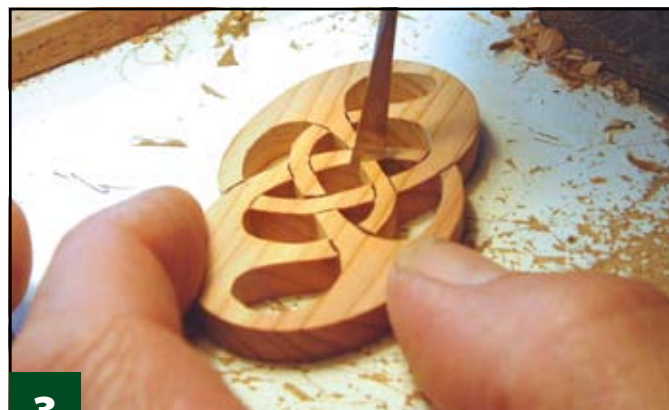
3 Outline the crossover points. Mark the areas where the knotwork passes over or under another section. Make vertical cuts on these lines with a gouge.
